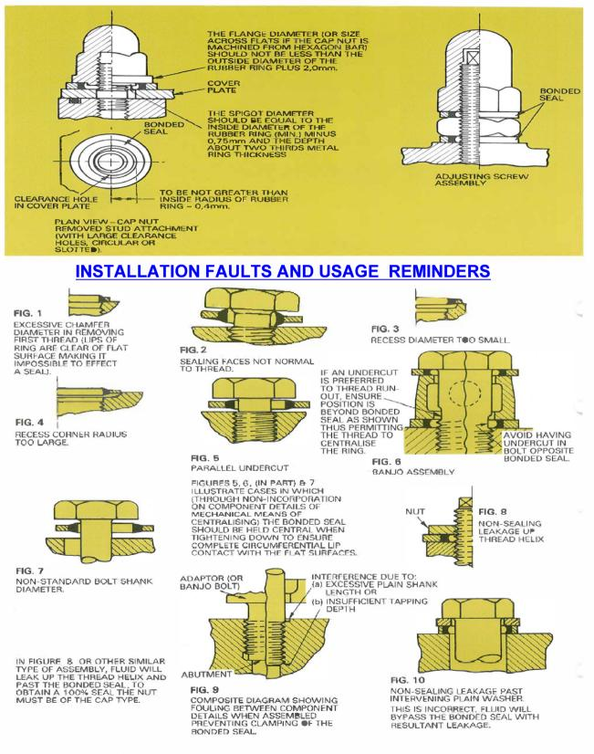
The above information will assist in the correct instalation and assembly of the bonded washers ensuring successfull application and service for pipes and fittings to the correct advised pressures .
